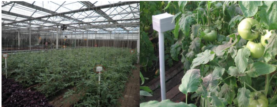
Figure 3. The sensor nodes deployed in the greenhouse
