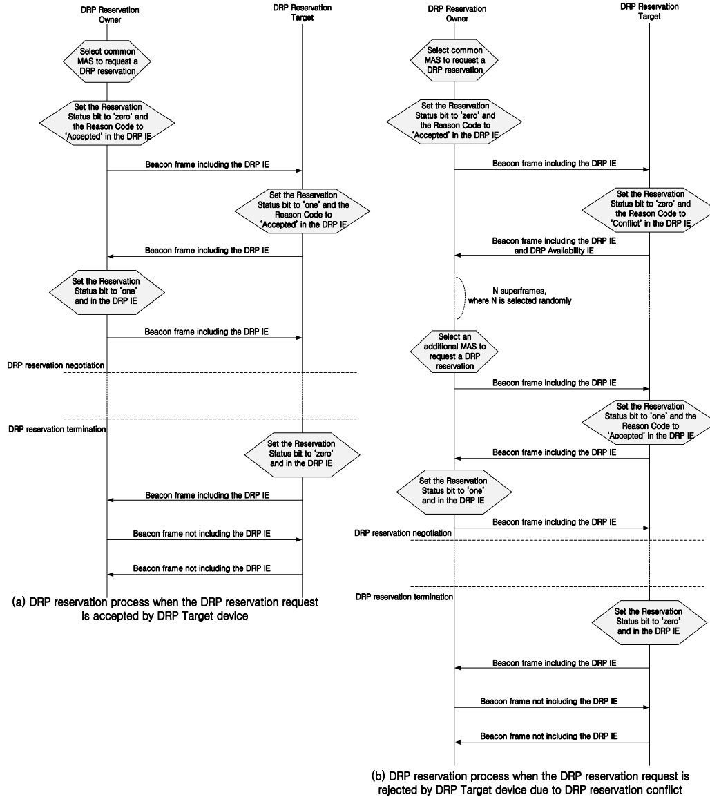
Figure 12. The inter-operation of RFID DRP negotiation
