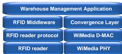
Figure 2. Protocol Layer Structure of RFID reader node combined with WiMedia D-MAC
