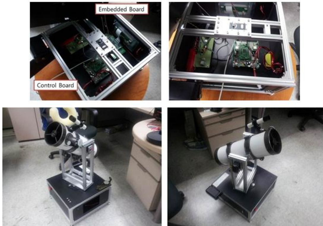
Figure 3. Our Implementation: Telescope Mounting System and its Control Module
