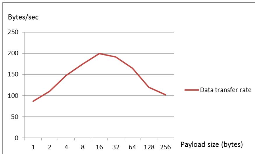
**Figure 5. Bluetooth Data Transfer Rate vs. APDU Payload**
