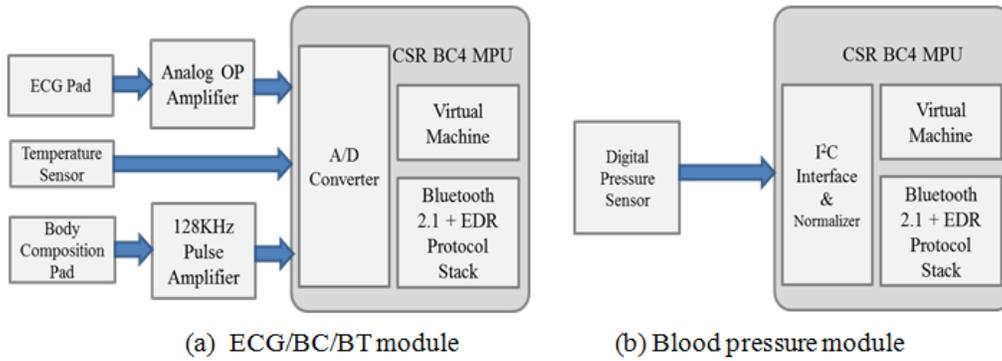
**Figure 2. The Block Diagrams of the Multifunction Module and BP Module**
