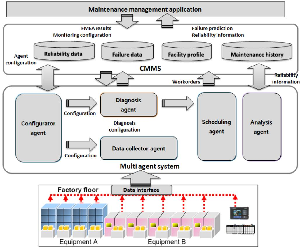
**Figure 2. System Architecture**
