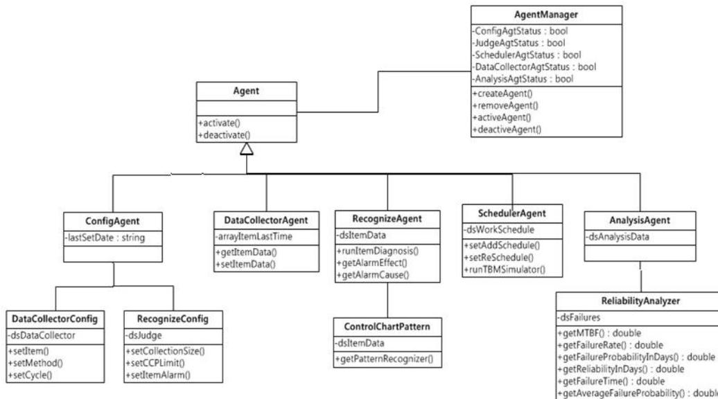
**Figure 1. Class Diagram; Agent Manager and Five Agent Types; configure, data collector, recognizer, scheduler, and analyzer**
