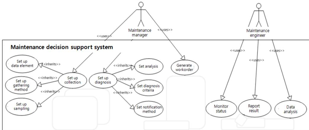
**Figure 3. Decision Support Scenario; a Use Case Diagram**
