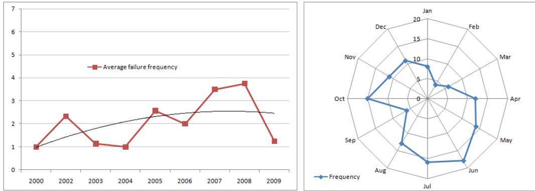
**Figure 5. Failure Pattern of Large Type Machines; a) Annual Failure Frequency, b) Seasonal Trend**
