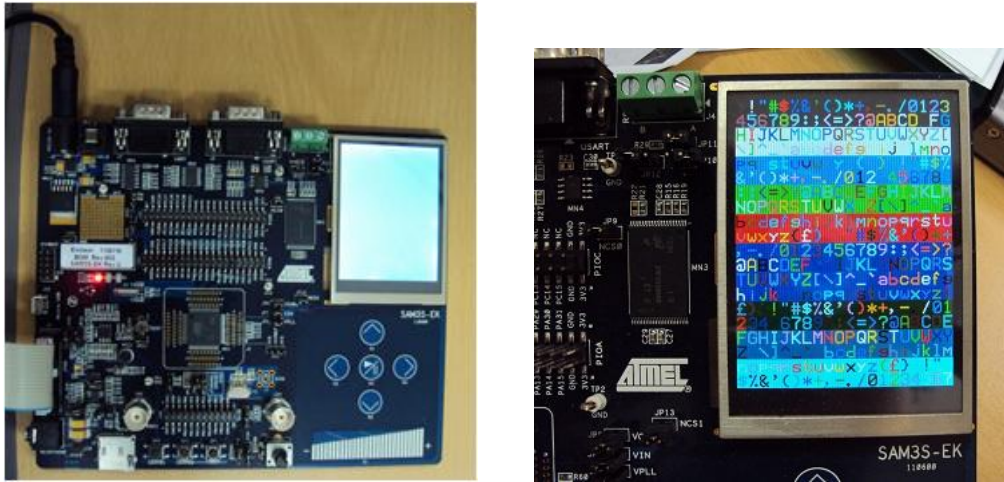
(a) an embedded board with an LCD display (b) the LCD display with 240x320 pixels
