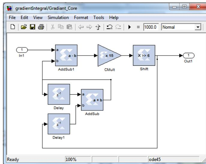
Figure 5. Algorithm Detail
