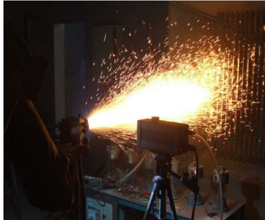
Figure 10. SprayWatch Thermal Spraying Jet Flow Inspection Device
