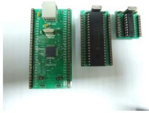
Figure 21. PIC Chip Example that is in the Kit ( PIC18F6627 ).
