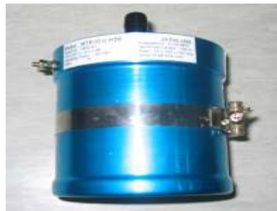
Figure 3. A photograph of the inductive coupler of the system
