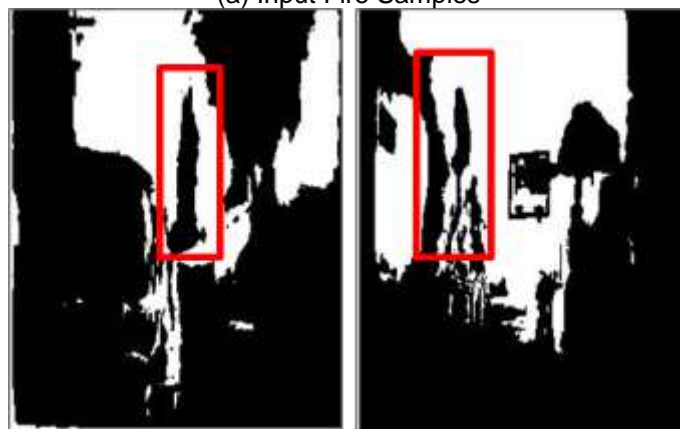
(b) Color Segmentation output using YCbCr
