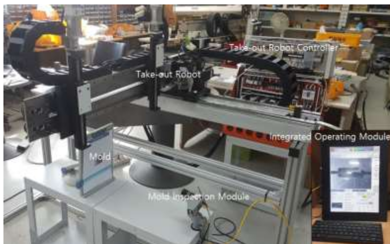
Figure 10. Experimental Setup for the Performance Test of Developed Take-out Robot Integrated Control System
