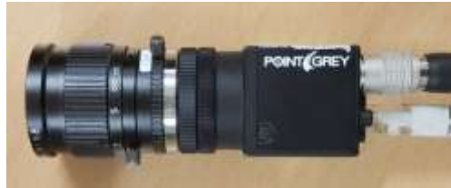
Figure 7. IP Camera Used in Mold Inspection Module
