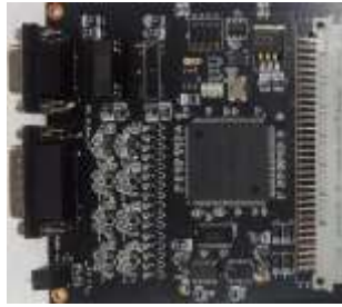
Figure 9. Developed Process and Peripheral Data Acquisition Interface Module
