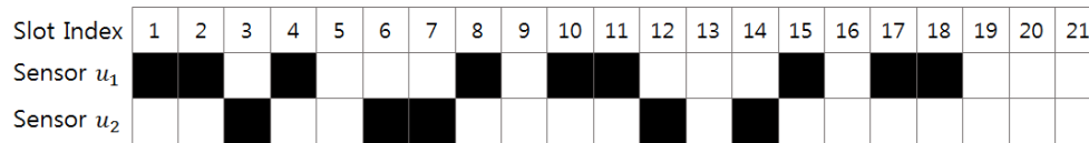
Figure 3. An Example of Two Asymmetric BIBD-based Schedules without any Common Active Slot
