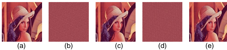
Figure 1. Arnold Transformation by using Different Times of n_e and n_d . (a) Plain-Image Lenna(512*512); (b) cipher-image n_e=100 ; (c) decipher-image (b), n_d=284 ; (d) cipher-image n_e=50 ; (e) decipher-image of (d), n_d=50
