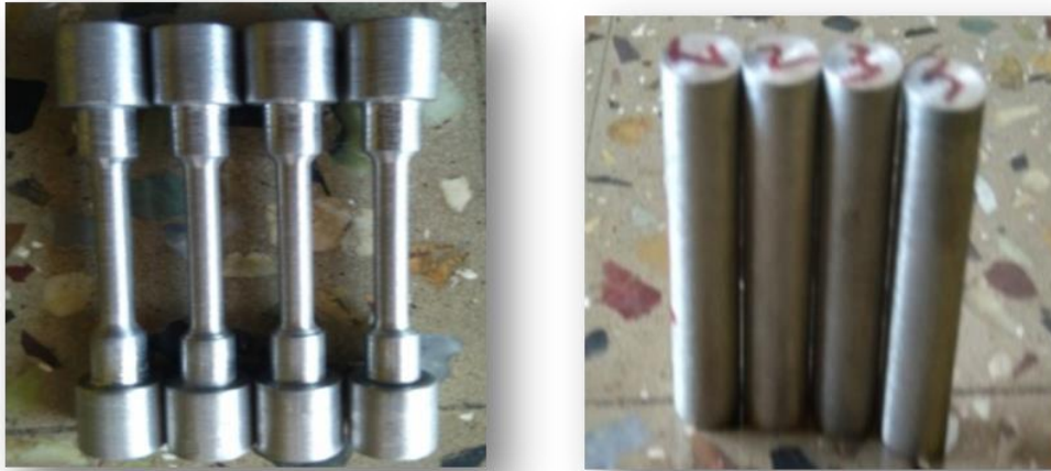
Figure 1. Tensile and Compression Test Specimens as per ASTM Standards
