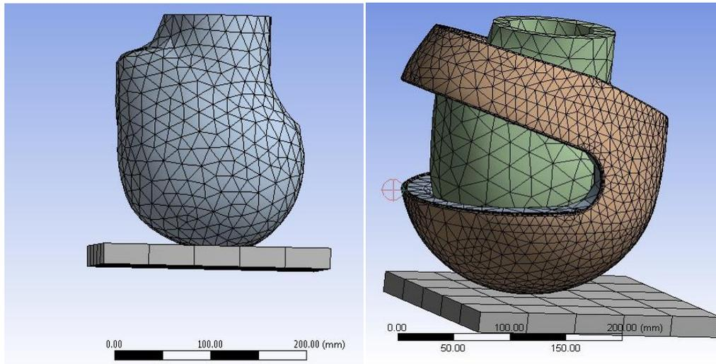
**Figure 5. Meshed Model of HF without (left) and with Helmet (right) in Crown Impact**
