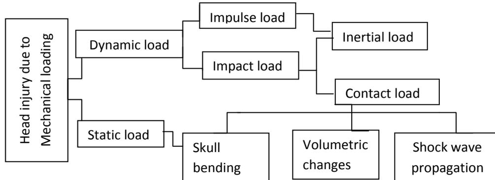
**Figure 1. Types of Load Act on Head Subjected to Collision**
