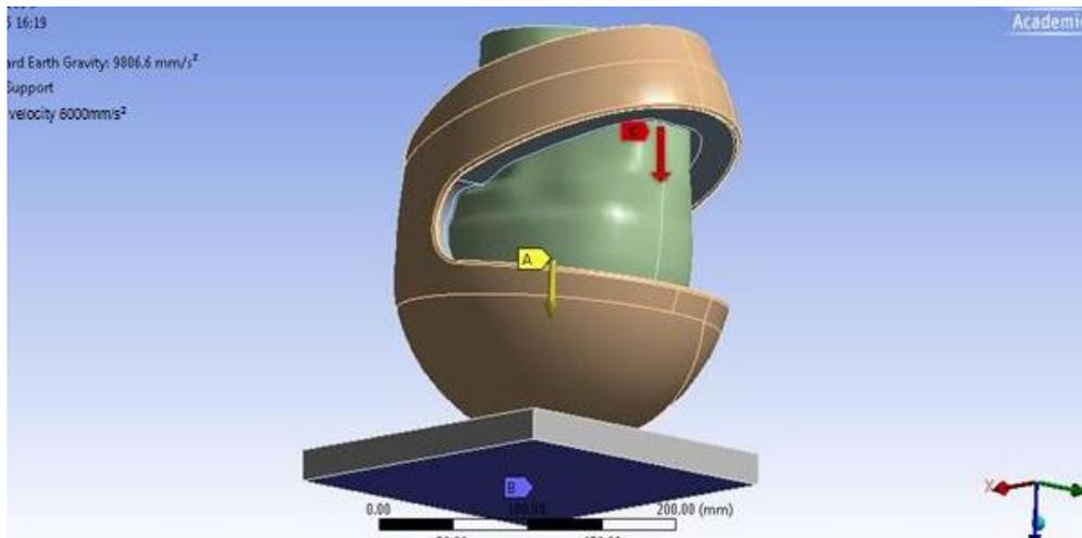
**Figure 7. Representation of Forces on HF-helmet Assembly**
