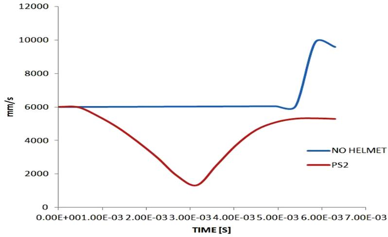
Figure 9. Velocity of Head Form with and without Helmet
