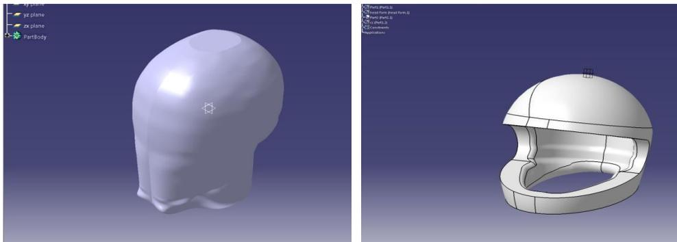
**Figure 3. Model Head Form (G) and Model of the Impact Absorbing Liner**
