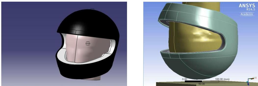
**Figure 4. Assembly of Head form and Helmet (Left) and Imported to ANSYS (right)**
