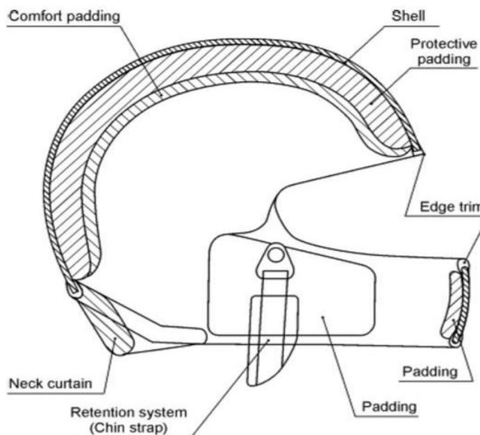
**Figure 2. Components of Typical Motorcycle Helmet**
