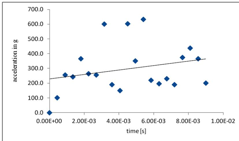
Figure 11. PLA of Headform with PS3 Liner in Crown Impact
