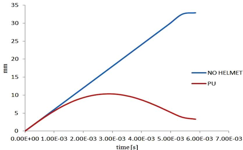
Figure 8. Deformation of Head Form with and Without Helmet
