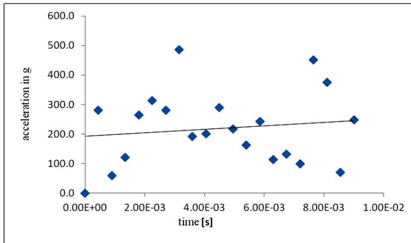
Figure 10. PLA of Headform with PS2 Liner in Crown Impact
