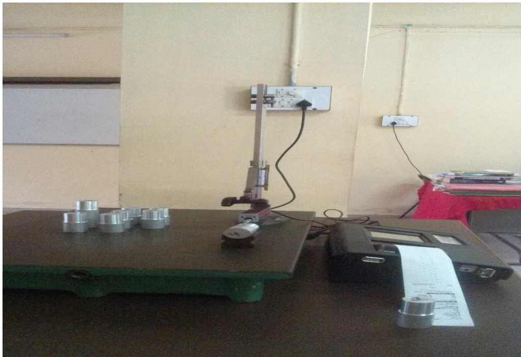
Figure 4. Experimental Setup for Measuring Surface Roughness
