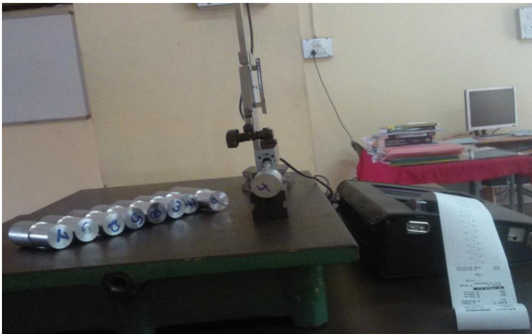
Figure 4. Surface Roughness Measurement Setup
