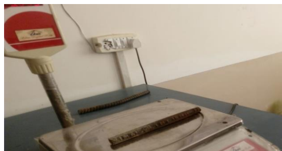
Figure 6. Weight of Steel Bar taken by Advance Digitally Weighing Machine
