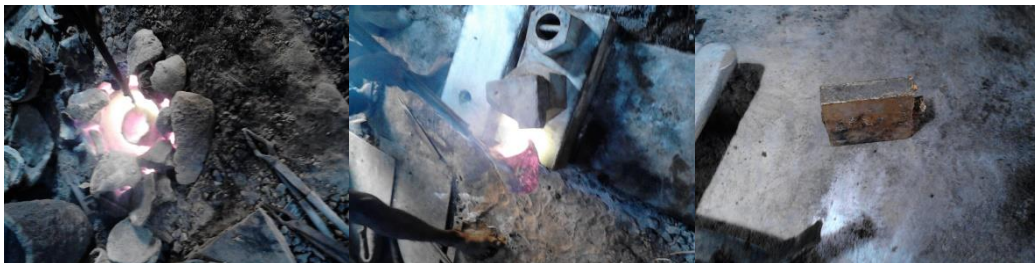
Figure 4. (a) Melting of Molten Metal (b) Pouring of Molten Metal (c) Final Casting Piece
