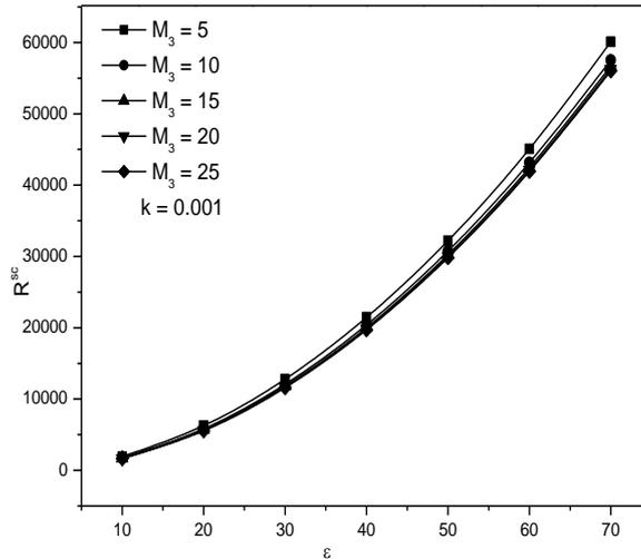
**Figure 5. Variation of  $R^{sc}$  versus  $\varepsilon$  for Different  $M_3$  with  $S_T = -0.002$ ,  $R_S = -500$ ,  $T_a = 10$  and  $\tau = 0.03$ .**
