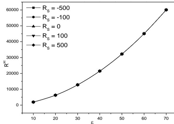
**Figure 2. Variation of  $R^{sc}$  versus  $\varepsilon$  for Different  $R_s$  with  $S_T = -0.002$ ,  $M_3 = 5$ ,  $k = 0.001$ ,  $T_a = 10$  and  $\tau = 0.03$ .**
