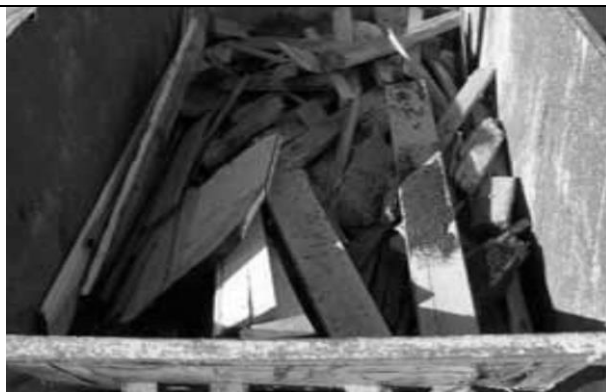
Figure 1. Wood Separated from Demolition Waste
