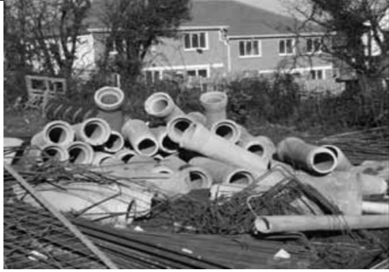
Figure 3(a). Construction and Demolition Waste – Source Separated
