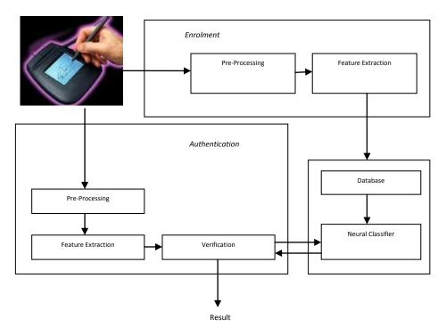
Figure 2. System Architecture
