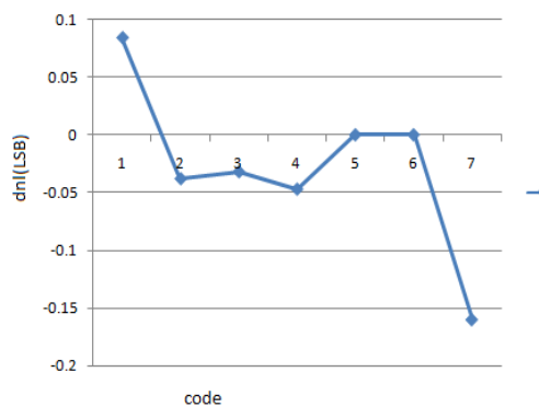
Figure 12. DNL Curve of Flash Type ADC using TMCC and Bit Referenced Encoder
