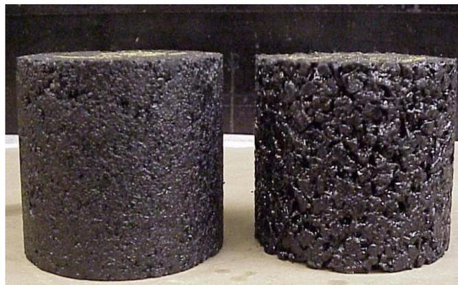
**Figure 4. Asphalt-cement and asphalt-cement-hair mixtures**
