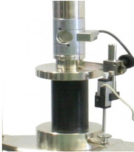
**Figure 5. Compressive Test**
