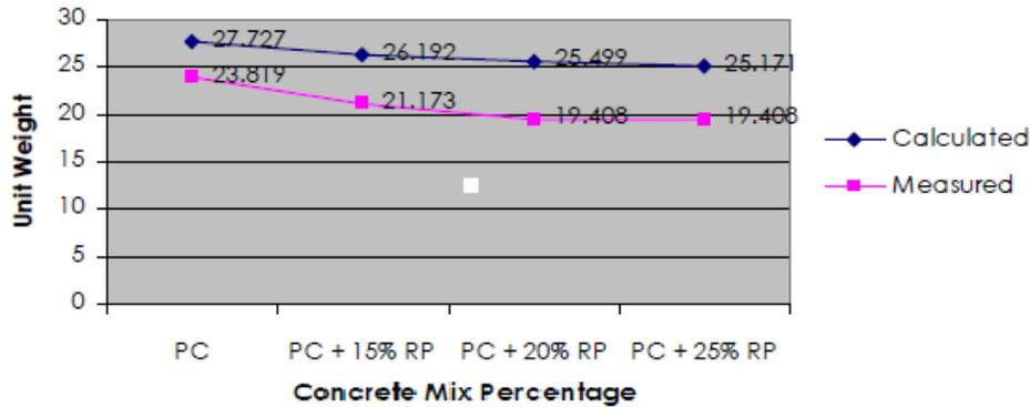
**Figure 1. Unit weight of cylindrical specimens**
