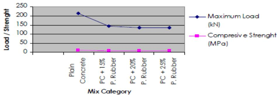
**Figure 2 . Compressive strength of specimens (concrete with pelletized rubber)**
