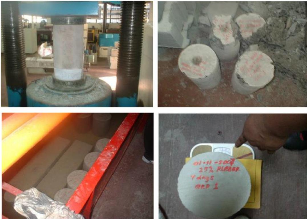
**Figure 3. Preparation of concrete cylindrical specimens with 25% with cut rubber pellet composition**
