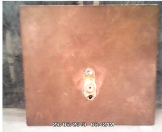
Figure 6. Bottom view of fabricated re-configurable fractal antenna
