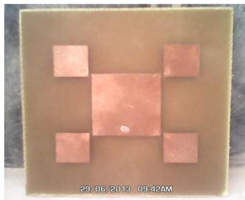
Figure 5. Top view of fabricated reconfigurable fractal antenna
