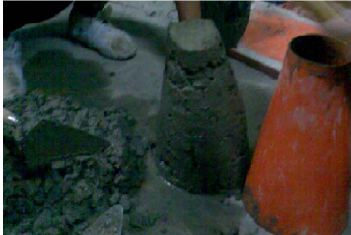
Figure 4. Slump testing the concrete mixture
