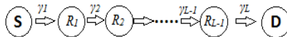
Figure 1. Schematic of a multihop network with source S is transmitting towards destination D via N-1 intermediate relays
