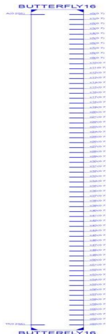
Figure 4.1. RTL View of a Butterfly Component Used In 256-Point FFT
