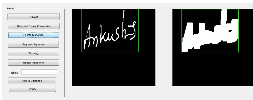
Figure 5. Proposed ROI Detection Technique to Solve Disconnected Signature Problem
