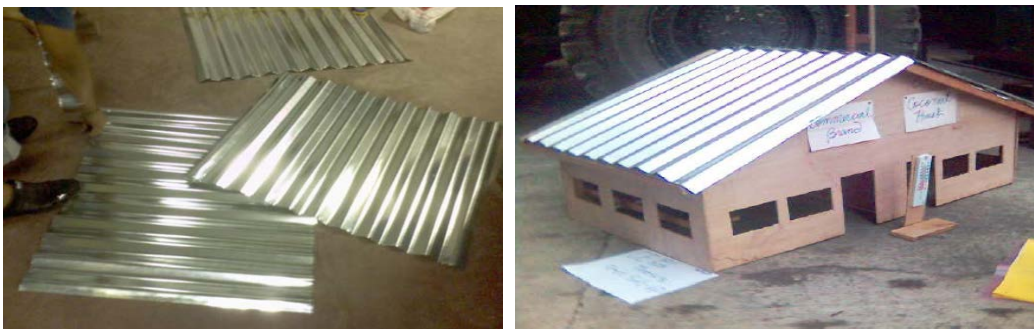
Figure 6. (a) Corrugated Roof Simulate Actual Roof Heat Absorption and (b) Regular Reading of Inside and Outside Temperatures on a 30 min. Interval
