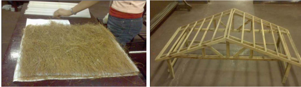
Figure 5. (a) Coco Coir Placement and (b) Truss Frame of the Heat Insulation Test Apparatus
