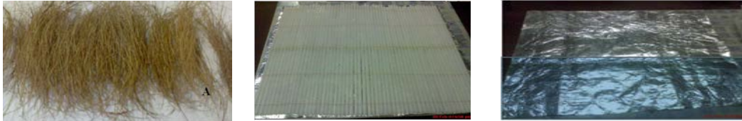
Figure 1. (a) Coco Coir Fibers. (b) Polypropylene Straws Threaded Together (75cm x 71cm) and (c) Aluminum foil (75cm x 71cm)
