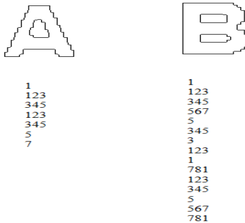
Figure 6. Standard DCC's of some English Alphabets, Saved in the Text Feature Database
