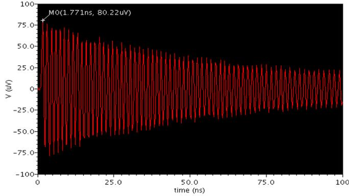
**Figure 9. Showing Ground Bounce Noise of Flash ADC**
