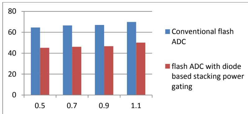
**Figure 7. Active Power Dissipation of 3 Bit Flash ADC**
