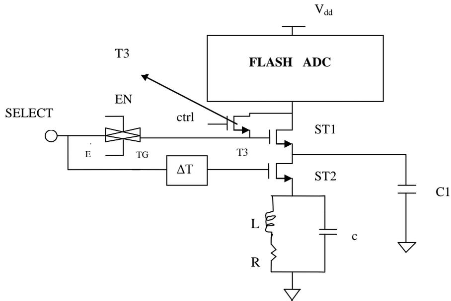
**Figure 4. Flash ADC Design with Diode based Stacking Power Gating Technique**
