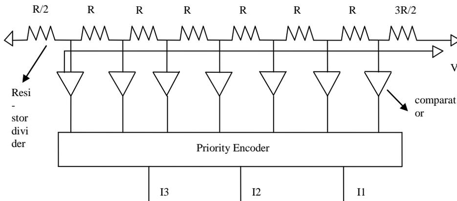
**Figure 1. Conventional flash ADC architecture [17]**
