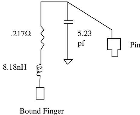
**Figure 8. DIP-40 Package Pin Ground Bounce Noise Model**
