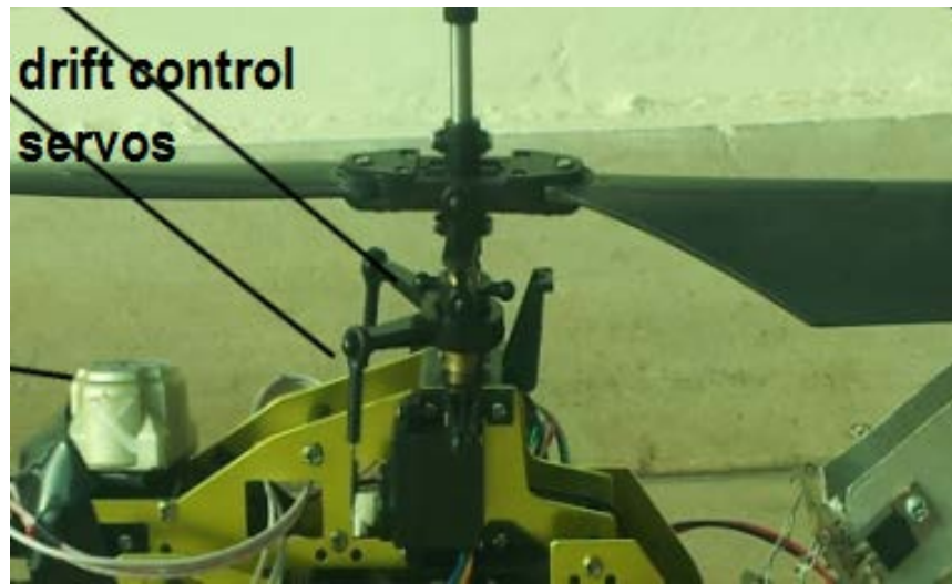
Figure 13. Horizontal Drift Control System
