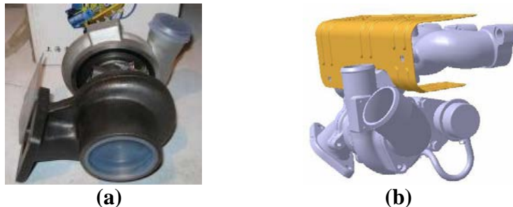
Figure 3. Turbochargers: (a) CARRETT; (b) MHI TD03 (with a Small Cross-Section and an Intercooler)
