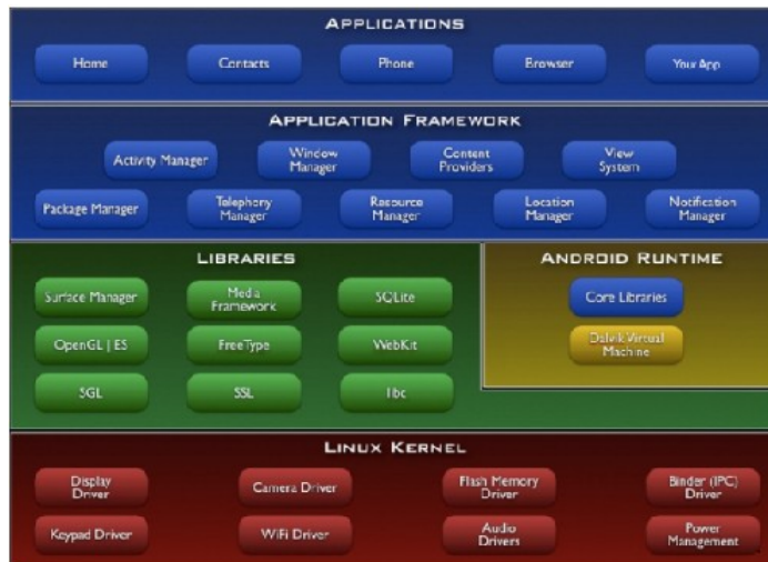
Figure 1. Android Software Stack [3]
