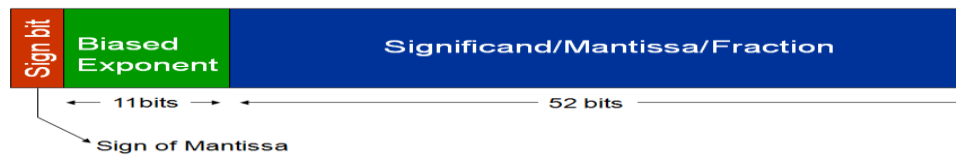
Figure 1. IEEE-754 double precision floating point format
