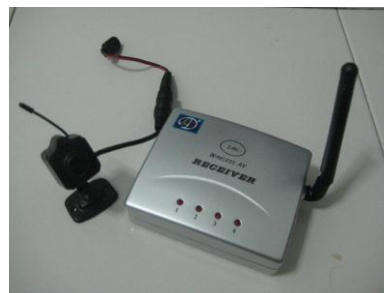
Figure 5. Wireless Camera and Receiver
