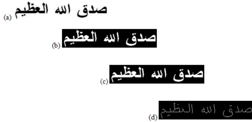
Figure 3. Preprocessing Steps: (a) input, (b) binary, (c) spurred, and (d) thinned
