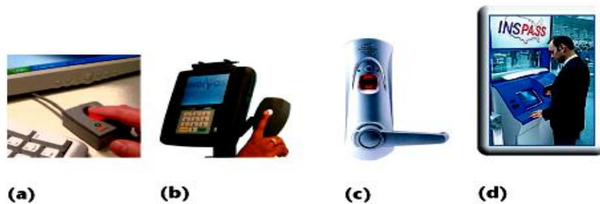
Figure 22. Biometrics Application Examples. (a) Digital Persona's fingerprint verification system provides personal recognition for computer and network login. (b) Indivos manufactures a fingerprint based point-of-sale (POS) terminal that verifies customers before charging their credit cards. (c) BioThentica's fingerprint-based door lock restricts access to premises. (d) The Inspass immigration system, developed by Recognition Systems and installed at major airports in the US, uses hand geometry verification technology [62].
