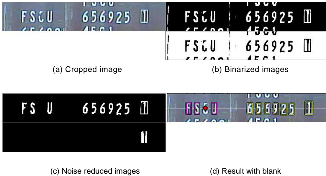
Figure 7. Character Extraction using Binarization
