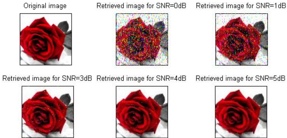
Figure 5. Transmitted and retrieved color images for user #1 under implementation of Minimum Mean Square Error (MMSE) signal detection technique in BPSK digital modulation at different Signal-to-Noise ratio (SNR)
