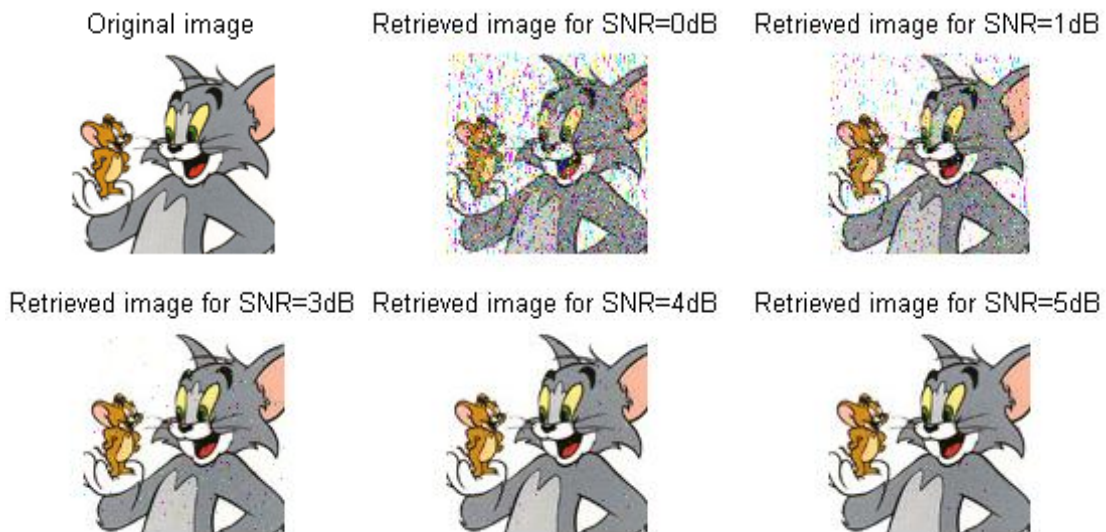
Figure 6. Transmitted and retrieved color images for user #2 under implementation of Minimum Mean Square Error (MMSE) signal detection technique in BPSK digital modulation at different Signal-to-Noise ratio (SNR)
