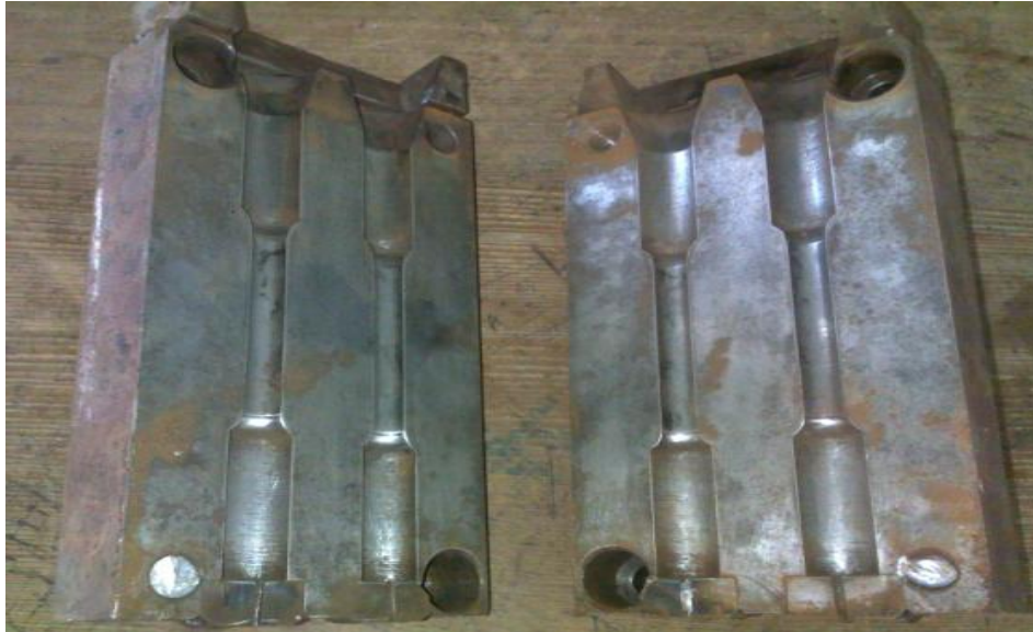
Fig5: Die for Tensile Test Specimens
