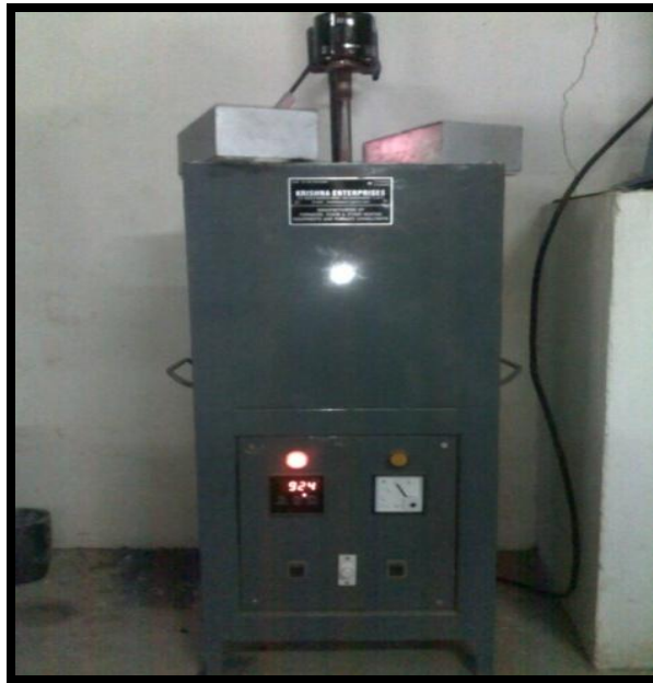
Fig 2: Electric Furnace with Mechanical Stirrer
