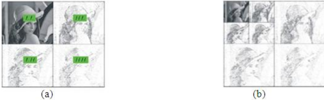
Figure 3: (a) One level wavelet transform in both directions of a 2D signal; (b) Two levels of wavelet transform in both directions
