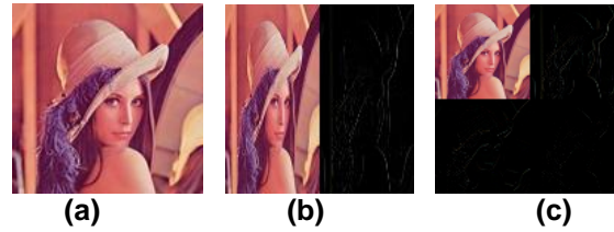
Figure 3. Non-standard Decomposition of an Image (a). Original image, (b). Decomposition of the row (c). Decomposition of the column
