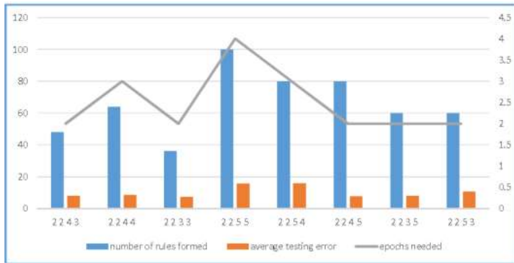
Figure 7. Comparison of Average Error Rates, Number of Rules Formed and Epochs Needed for Different Number of Membership Functions
