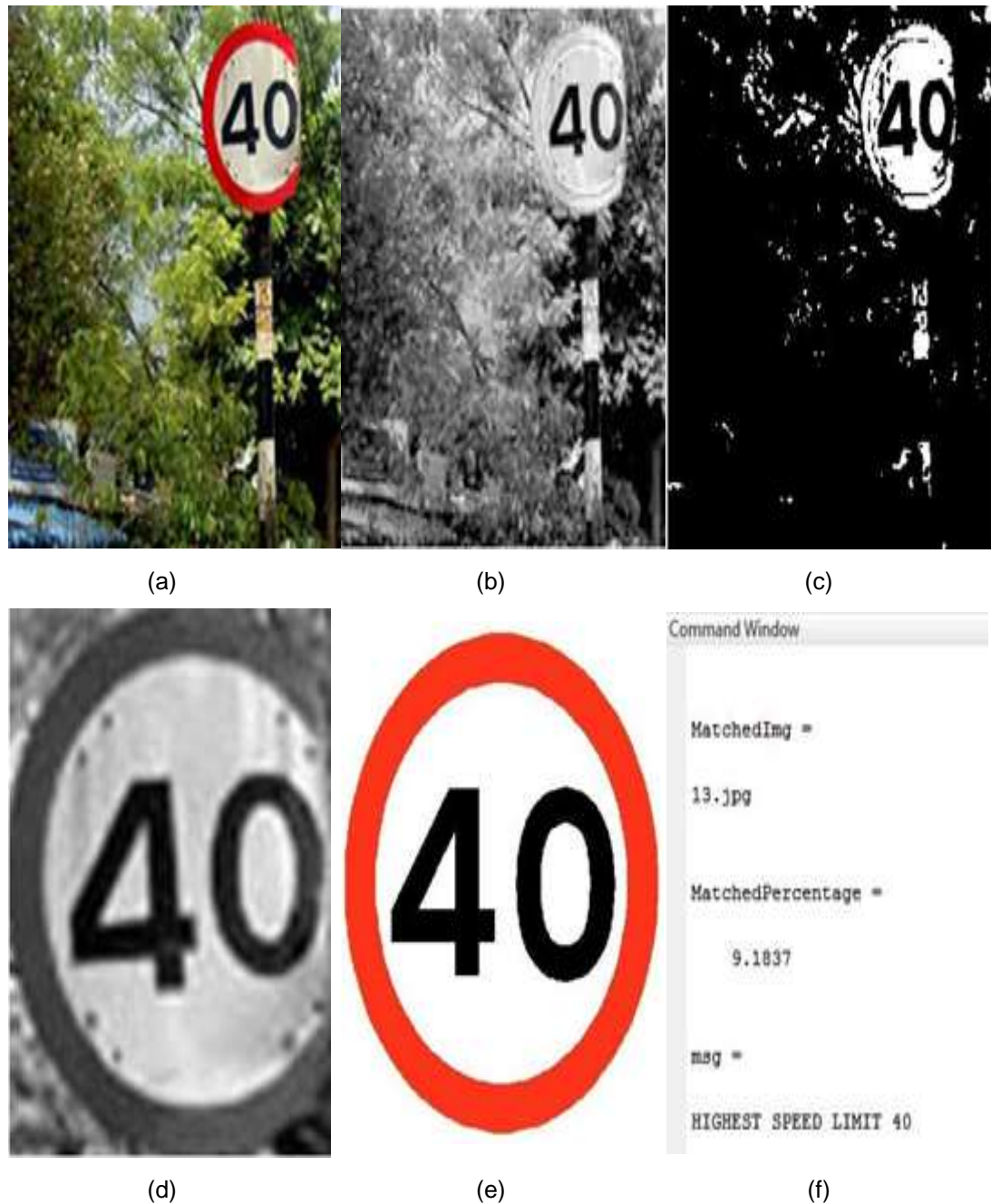
Figure 6. (a) Input RGB Image, (b) Input Image after Red Channel Extraction, (c) Binary Image, (d) Detected Road Sign (e) Recognized Road Signs, and (f) Meaning of Road Signs in the Command Window
