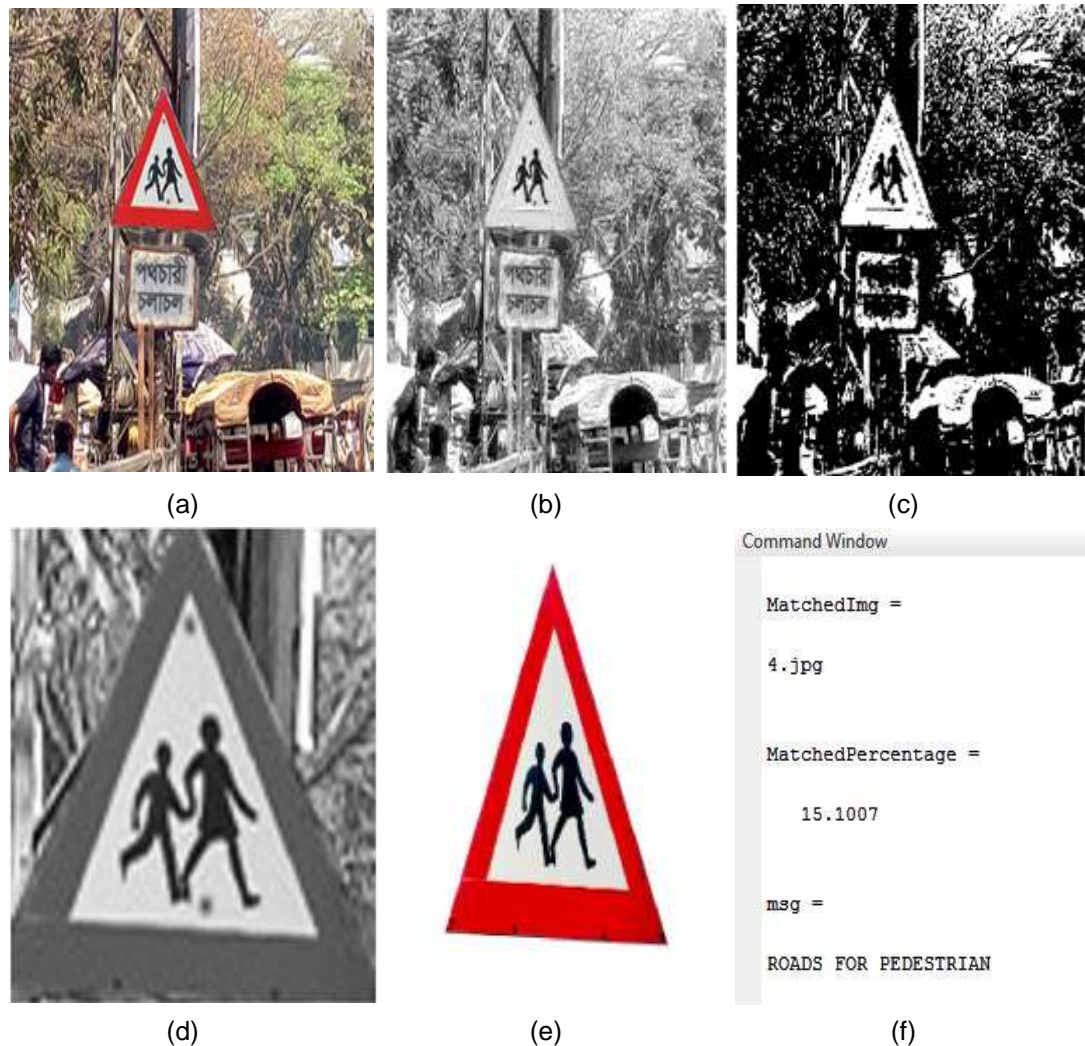
Figure 5. (a) Input RGB Image, (b) Input Image after Red Channel Extraction, (c) Binary Image, (d) Detected Road Sign, (e) Recognized Road Signs, and (f) Meaning of Road Signs in the Command Window
