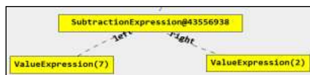
Figure 5. Changing the Name of an Object through toString() Overriding
