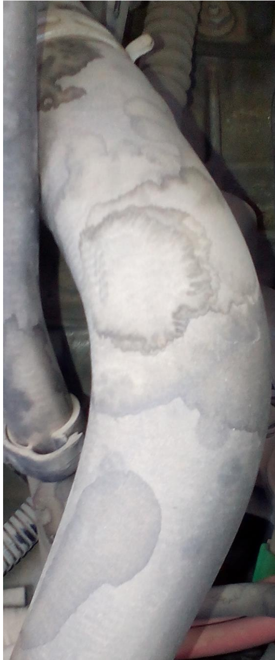
Figure 6. False Positive Case of an Unflawed Pipe
